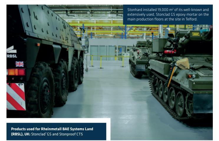
Single-source industrial flooring specialist Stonhard has met one of its heaviest-duty challenges in years by laying a high performance, power-trowelled epoxy floor mortar to withstand traffic from 70 tonne tanks manufactured by a Shropshirebased defence engineering company.
